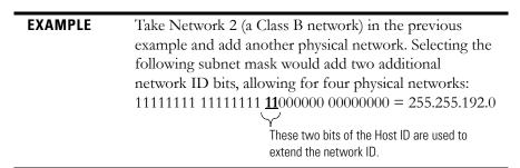
Two bits of the Class B host ID are used to extend the network ID. Each unique combination of bits in the part of the Host ID where subnet mask bits are 1 specifies a different physical network.
