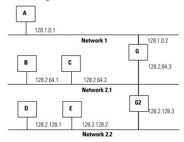
A second network with Hosts D and E was added. Gateway G2 connects Network 2.1 with Network 2.2.
