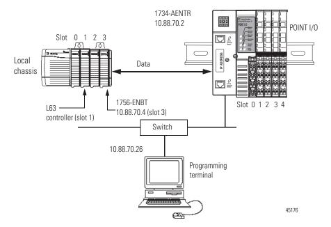
To work along with this example, set up your system as shown in the figure.
