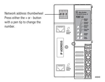
The adapter reads the thumbwheels first to determine if the thumbwheels are set to a valid number. You set the node address by using the 3-position pen-push thumbwheel using a pen tip.
